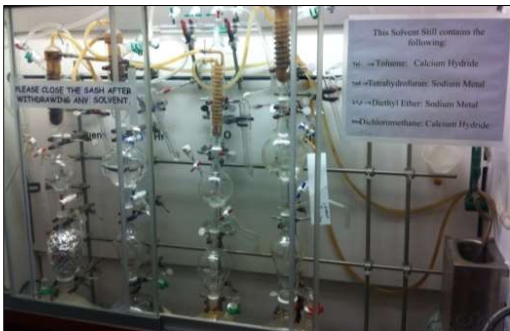
Figure 4.2 – Alternative Labeling of Chemical Fume Hood Reaction Vessels
