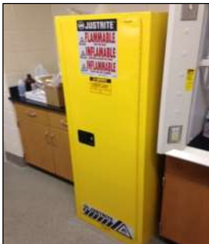
Figure 5.1 – Flammable Storage Cabinet
